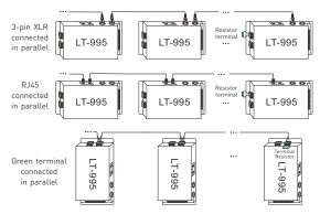
These 3 terminals can be connected in a mixed way.
