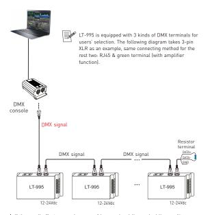
\* If the recoil effect occurs because of longer signal line or bad line quality, please try to connect 0.25W 90-120 $\Omega$  terminal resistor at the end of each line.
